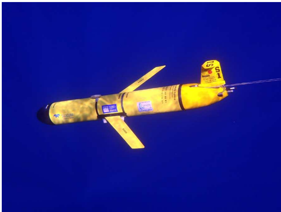
125 Figure 1. The SLOCUM G2 glider during the ABACUS pre-mission test at sea. Credit M. Torner.
