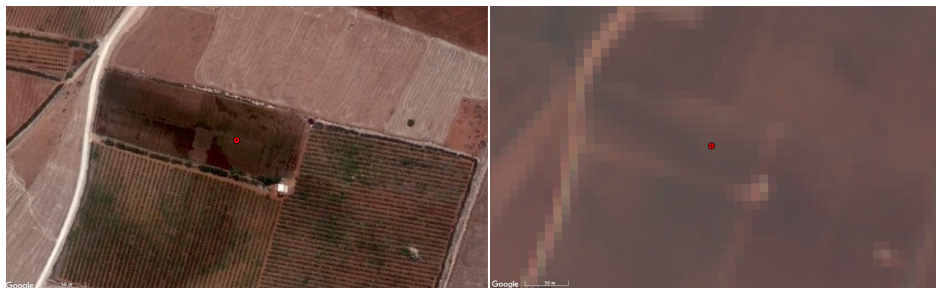
Fig. 1. Illustration of the level of detail that users can detect. Figure on the left: a VHR image from Google Maps. Figure on the right: a Sentinel-2 image (natural colors) at 10 m resolution.
