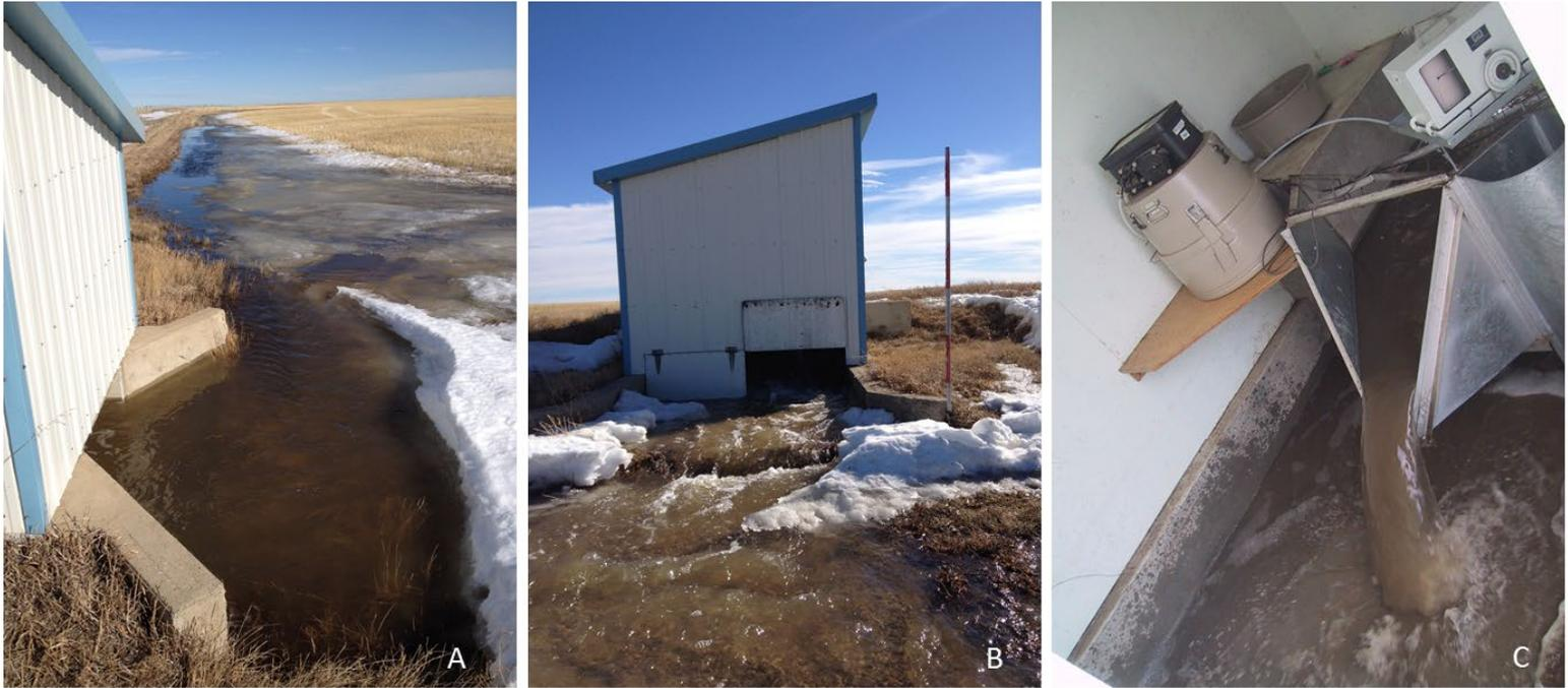
**Figure 3.** Photographs of the runoff shed at Hillslope 2. A) Facing east, at the inflow side of the shed (taken March 2014). B) Facing south, at the outflow side of the shed (taken March 2014). C) Inside the shed, showing a 0.61m H flume, a Stevens water level chart recorder, and an automated ISCO 3700 Portable Sampler.
