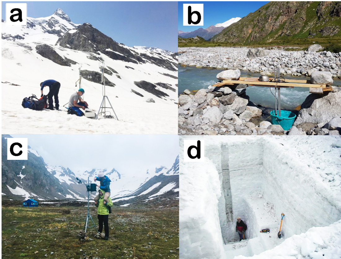
5 Figure 3: (a) Campbell meteorological complex with a set of Kip & Zonen radiometers and GILL three-component acoustic anemometer at the Djankuat GlacierAWS1 location; (b) the construction of the Djankuat Gauging Station; (c) Djankuat Base Camp AWS - Davis meteorological station; (d) Snow density measurement in a snowpit at the stake 49.
