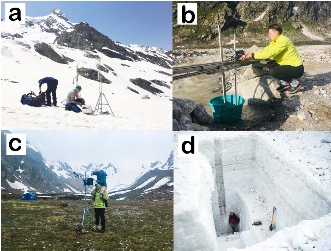
Figure 3: (a) Campbell meteorological complex with a set of Kip & Zonen radiometers and GILL three-component acoustic anemometer at the Djankuat GlacierAWS1 location; (b) the construction of the Djankuat Gauging Station; (c) Djankuat Base Camp AWS - Davis meteorological station; (d) Snow density measurement in a snowpit at the stake 49.
