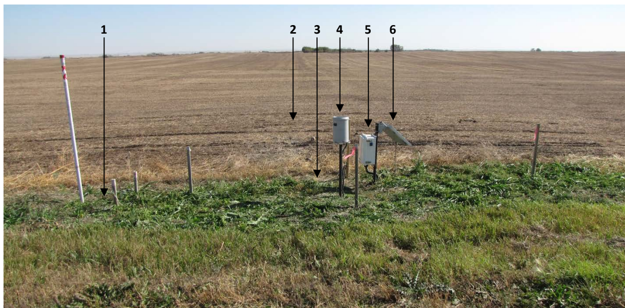
Figure 2. Typical site installation. (1) Horizontal 5 cm sensor; (2) horizontal 20 and 50 cm sensors and location of vertical 0-5 cm sensor during field season; (3) location of vertical 0-5 cm sensor during off season; (4) tipping bucket rain gauge; (5) loggerbox with datalogger; (6) solar panel.
