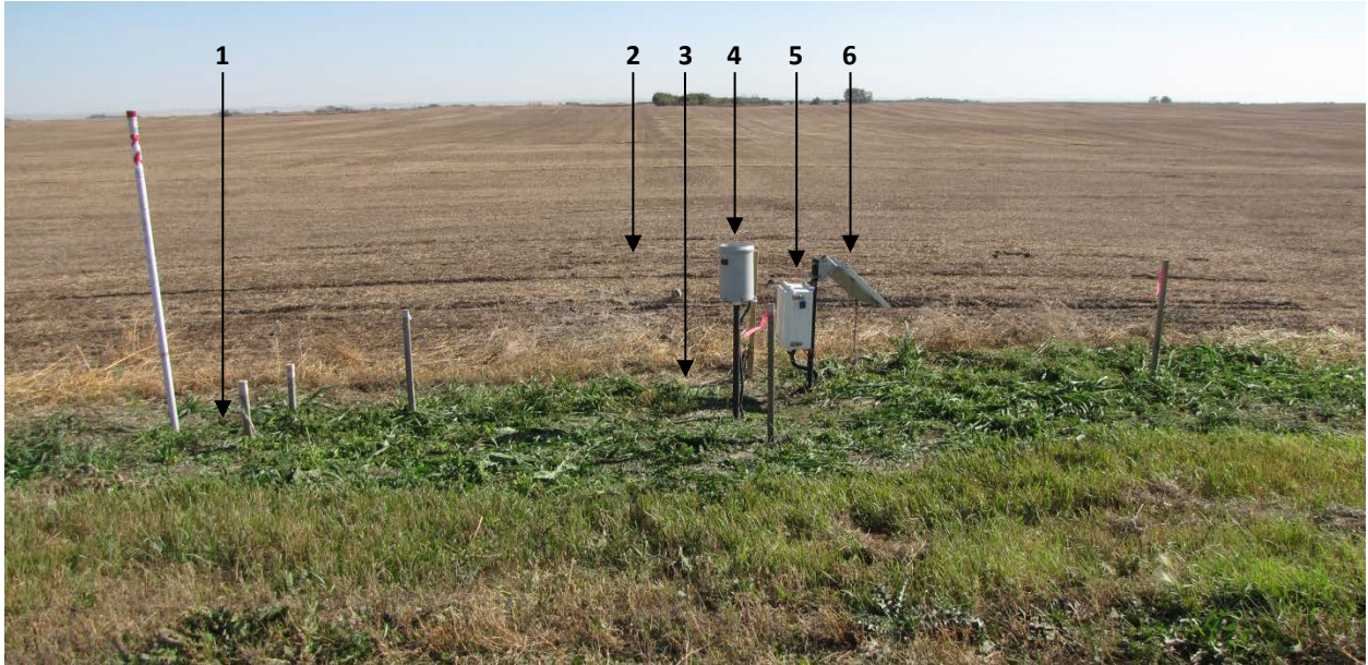
375 Figure 2. Typical site installation. The 4-probe sites include at (1) horizontal 5 cm sensor; (2) horizontal 20 and 50 cm sensors and location of vertical 0-5 cm sensor during field season; (3) location of vertical 0-5 cm sensor during off season; (4) tipping bucket rain gauge; (5) loggerbox with datalogger; (6) solar panel. Only ECCC sites have a vertically placed probe. The 3-probe sites are similar, with all probes located at the edge of field at (1).
