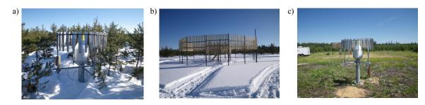
**Figure 4:** Precipitation gauge installations at the Caribou Creek SPICE site: a) Bush shielded Geonor T-200B with Alter shield, b) DFAR with Geonor T-200B in clearing and c) Alter shielded Geonor T-200B in clearing.
