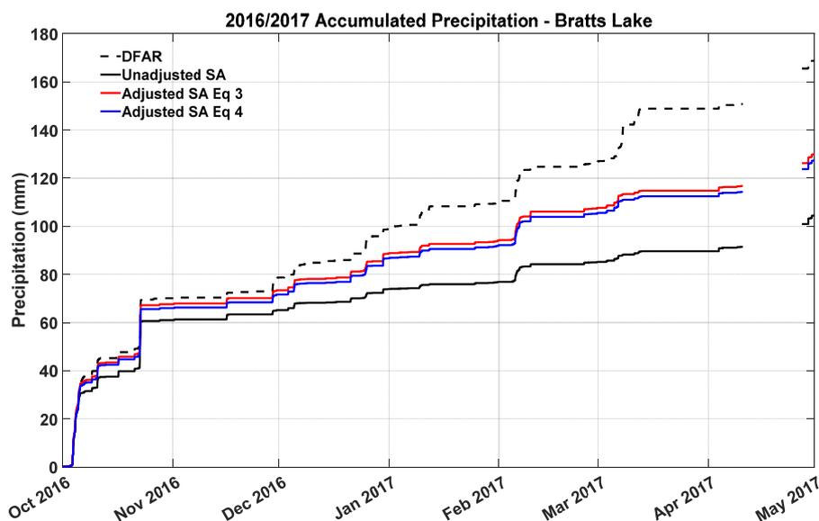
**Figure 7:** 2016/2017 winter accumulated precipitation time series from a) Caribou Creek and b) Bratt's Lake showing the unadjusted single Alter Geonor T-200B (solid black), the adjusted single Alter Geonor T-200B (red and blue solid; via the SPICE Eq. 3 and Eq. 4 transfer functions from Kochendorfer et al. 2017b), and the DFAR (dashed black).
