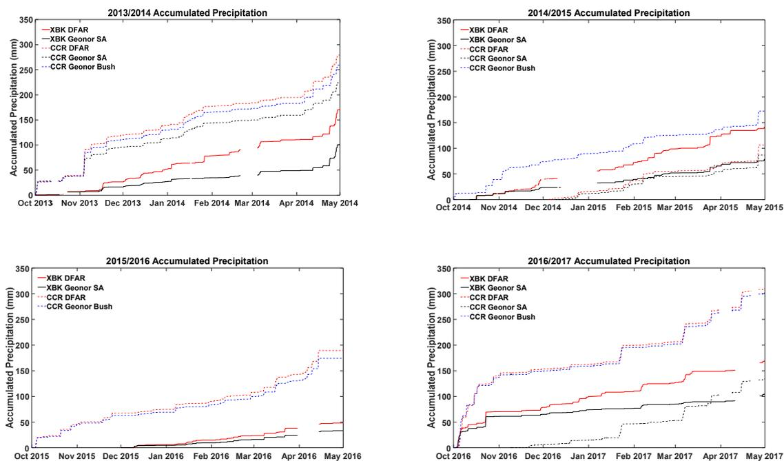
**Figure 5:** Seasonal time series of accumulated precipitation for the various gauge configurations at Bratt’s Lake and Caribou Creek. Note that although the accumulation season is from 1 October through 30 April, not all time series start at the beginning of the season due to gauge or site issues (see Table 2).
