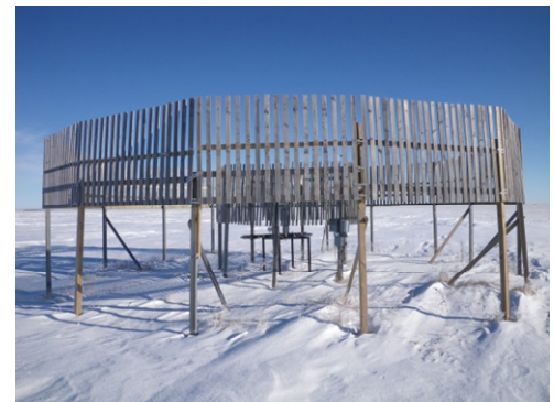
Figure 1: Conceptual diagram (left; Nitu & Roulet, 2016; diagram courtesy of Jeff Hoover, Environment and Climate Change Canada) and photo (right; Bratt's Lake) of the WMO DFAR.
