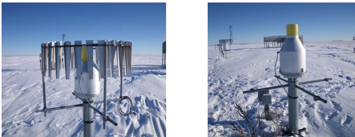
Figure 2: The SPICE Alter shielded (left) and unshielded (right) Geonor T-200B gauge pair at Bratt's Lake.
