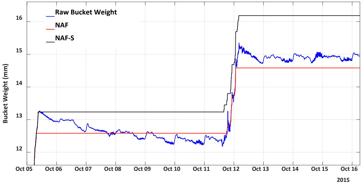
Figure 5: NAF (red) and NAF-S (black) precipitation data time series data processing example as compared to the Gaussian filtered raw bucket weight (blue). Data excerpt is from an actual precipitation time series observed at XBK in October 2015.
