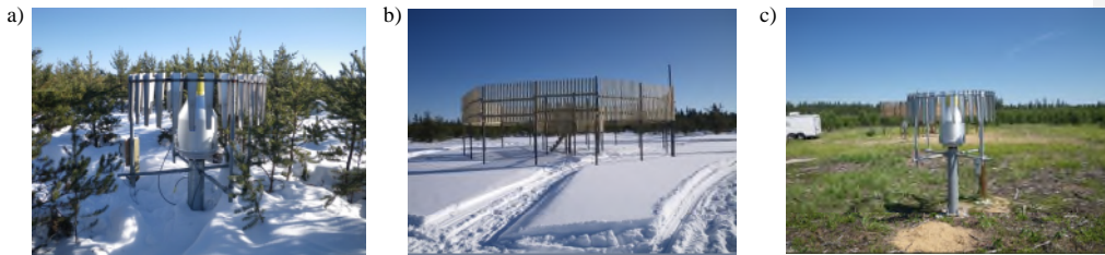
Figure 4: Precipitation gauge installations at the Caribou Creek SPICE site: a) Bush shielded Geonor T-200B with Alter shield, b) DFAR with Geonor T-200B in clearing and c) Alter shielded Geonor T-200B in clearing.
