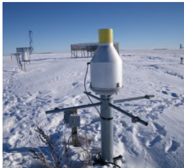
Figure 2: The SPICE Alter shielded (left) and unshielded (right) Geonor T-200B gauge pair at Bratt's Lake.
