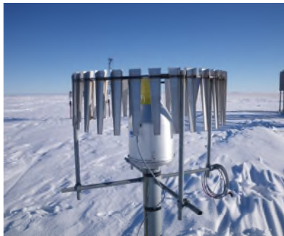
Figure 2: The SPICE Alter shielded (left) and unshielded (right) Geonor T-200B gauge pair at Bratt's Lake.
