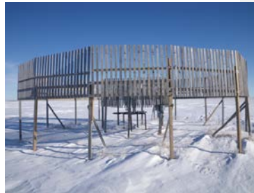
Figure 1: Conceptual diagram (left; Nitu & Roulet, 2016; diagram courtesy of Jeff Hoover, Environment and Climate Change Canada) and photo (right; Bratt's Lake) of the WMO DFAR.
