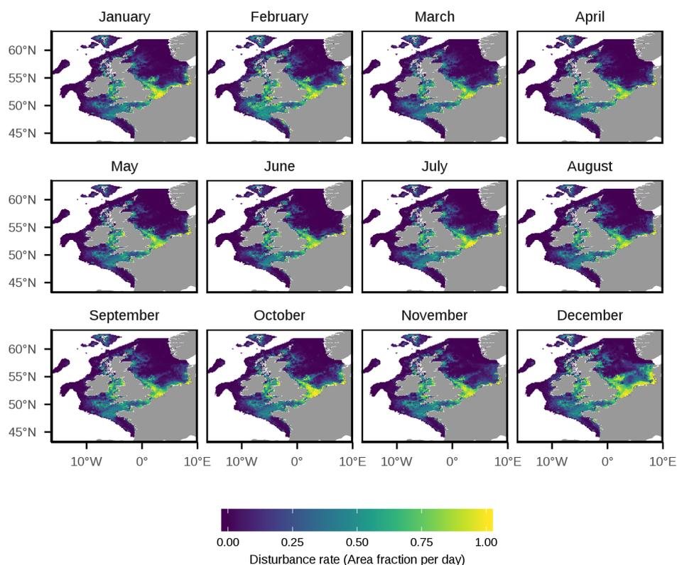
**Figure 10.** Modelled monthly disturbance rate. A disturbance event was defined as a time when the bed shear stress exceeded the threshold required to move either the mud, sand or gravel portion of the sediment. Monthly disturbance rate was defined as the mean fraction of the total mud, sand and gravel area disturbed per day.
