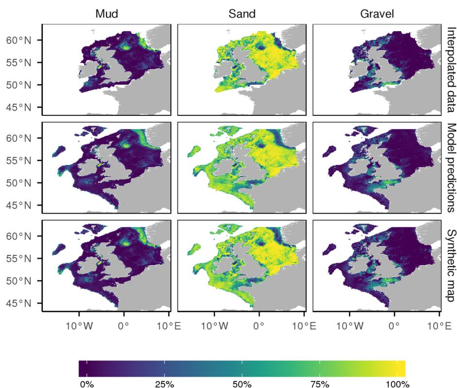
**Figure 4.** The derivation of the synthetic map of sediment percentages. The interpolated map uses bilinear spline interpolation using sediment data over the region. The random forest map predicts the sediment percentages using a random forest model which relates the percentage to the bed shear stress and the distance to the coast. The synthesized map merges the two, using spatial interpolations where we have data, and the random forest predictions where we do not.
