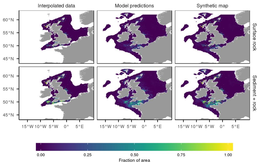
**Figure 8.** Proportion of area in each rock classification. Areas were classified by whether there was rock at the surface or a surface sediment layer plus rock in the top 50 cm. Historical survey logs and borehole records were first interpolated to provide a map of rock cover where we have sufficient data. Random forests were used to predict rock cover elsewhere using wave and tidal velocities, bathymetry, measures of bathymetry variation and distance from the coast as predictors.
