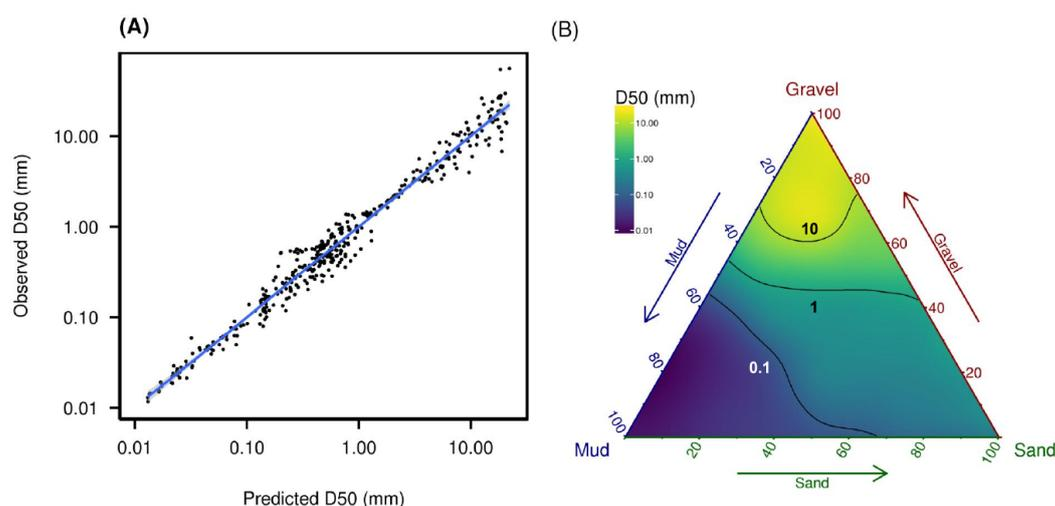
**Figure 5.** A: Predictions of a GAM model that relates whole-sediment D50 to the mud, sand and gravel percentages. B: Relationship between total sediment median grain size and percentage mud, sand and gravel. The relationship was derived using a general additive model which relates the D50 to the mud, sand and gravel percentage.
