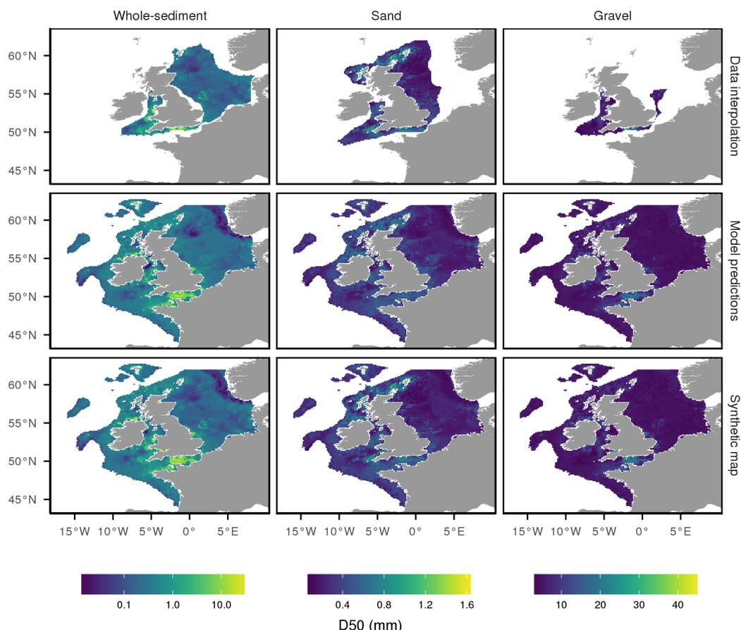
**Figure 6.** Summary of derivation of the synthetic median grain size maps. Where we have sufficient median grain size data we spatially interpolated a map of D50. In other locations we used the synthetic map of mud, sand and gravel percentages and a GAM model which relates the D50 to the mud, sand and gravel percentages to predict the D50.
