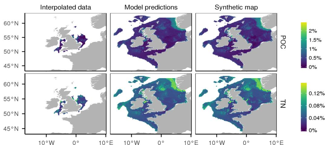
**Figure 9.** Derivation of the synthetic maps of particulate organic carbon (POC) and total nitrogen (TN) of sediments. Data was interpolated based on field observations in areas with good spatial coverage. In other regions, parameters were predicted using a random forest which had mud content and physical environmental variables as predictors.
