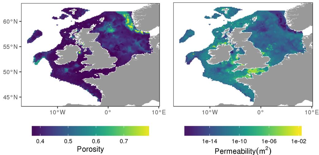
**Figure 7.** Maps of porosity and permeability. The relationship between porosity and permeability and median grain size was estimated using published field data. We then predicted porosity and permeability using the synthetic map of median grain size.
