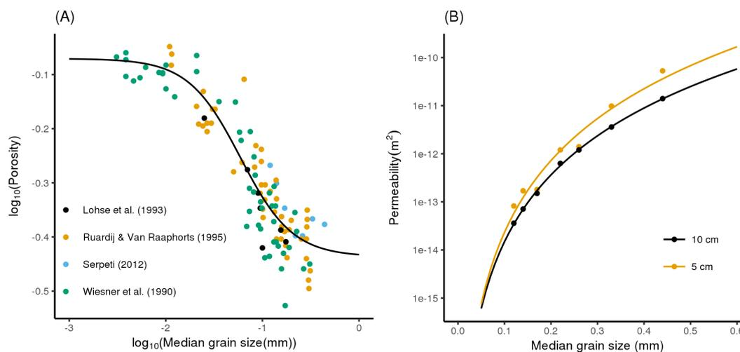
**Figure 3.** A: Assembled data on sediment porosity and median grain size (filled circles), and the fitted relationship (solid line). B: Annual average permeability  $\text{m}^{-2}$  of sediments from 7 sites off the north east coast of Scotland; Data from Serpetti (2015).
