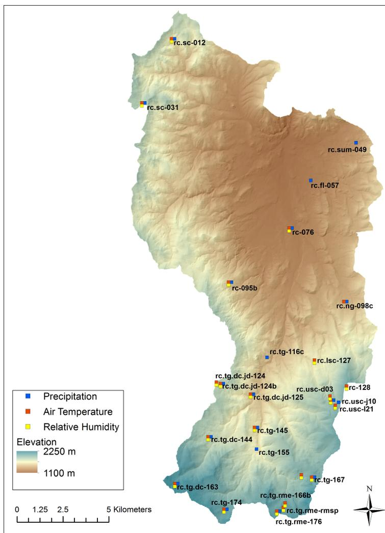
**Figure 1.** Location map of Reynolds Creek Experimental Watershed showing the elevation (m.a.s.l.) and the location of instruments used to measure precipitation, air temperature, and relative humidity.
