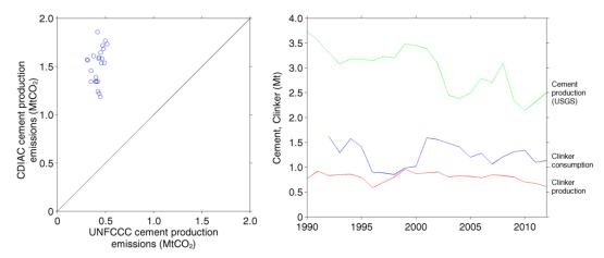
Figure 6: Netherlands. Left: CDIAC vs UNFCCC. Right: Clinker, cement. Note 'Clinker consumption' is production plus imports less exports, but excludes stock changes. Sources: (UNSD, 2015;UNFCCC, 2014;van Oss, 1994–2012;Boden et al., 2013).
