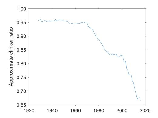
Figure 38: Implied global clinker ratio, derived from emissions estimates and cement production data.
