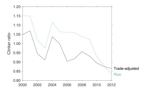
5 Figure 28: Indonesian clinker ratio, calculated from both clinker production and consumption data.
