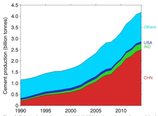
Figure 7: Global production of cement since 1990, highlighting the top-three producers, and showing the significant growth in China.
