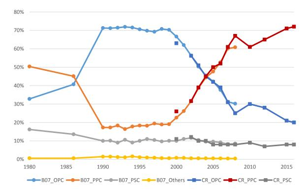
Figure 14: Proportions of cement production by type. B07: (J.D.Bapata et al., 2007), CR: (CRISIL, various years). OPC: Ordinary Portland Cement, PPC: Portland Pozzolana cement, PSC: Portland Slag Cement.
