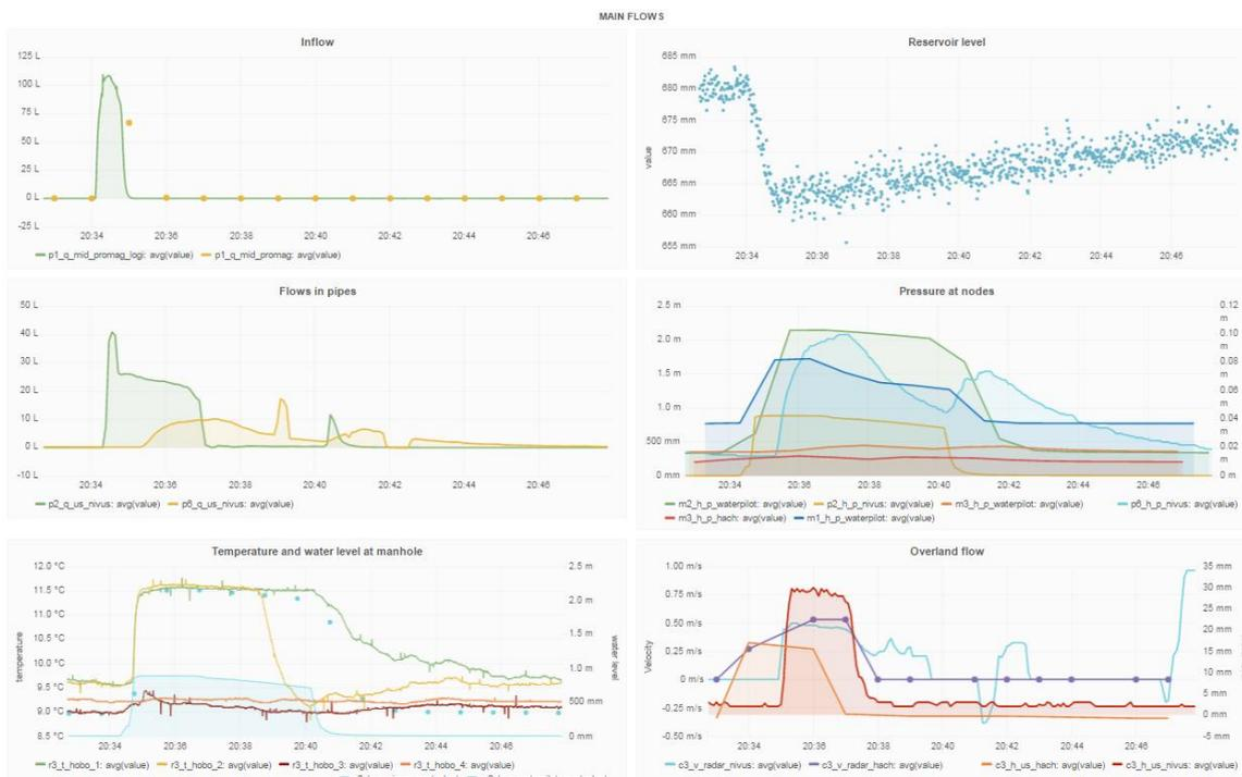
Figure 3: Extract of data for one experiment, for a selection of sensors. The hydrograph can be seen in the upper left chart in green.
