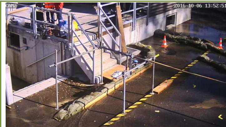
**Figure 1: View from camera CAM2 in which channel c3 is visible, as well as the scaffolding holding two radar-based flow measurement systems. The same channel is also visible from camera CAM3.**
