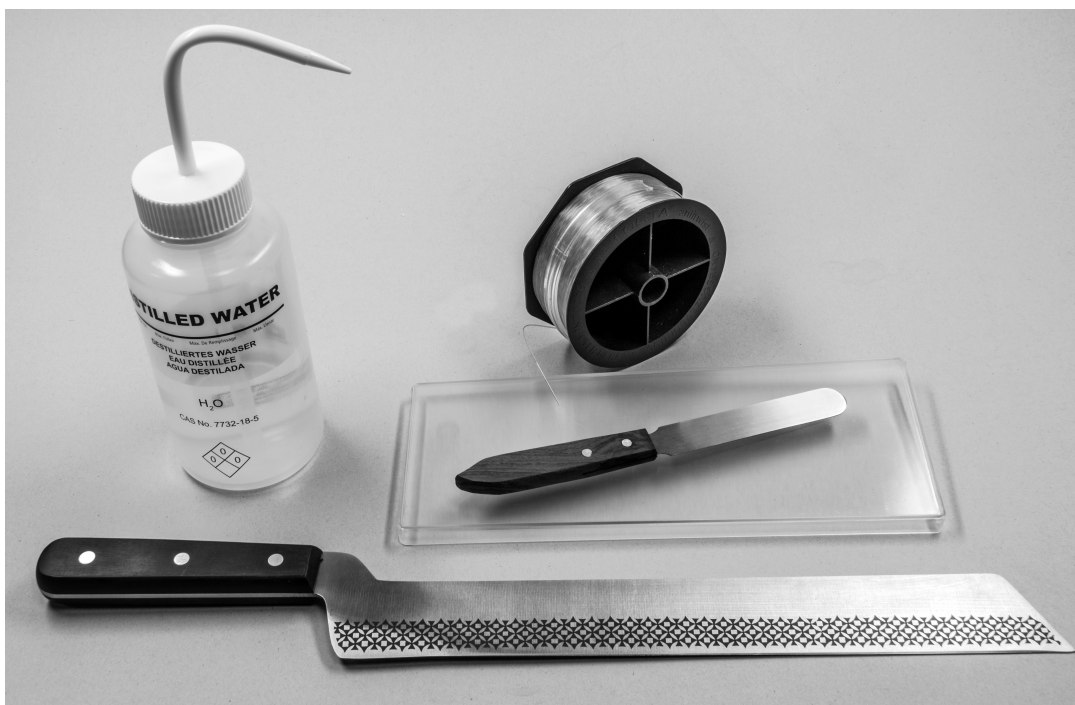
Figure 4: Equipment used for the preparation of sediment slabs for X-ray imaging comprise fishing line, distilled water, cheese knife, spatule and special Plexiglas lids for support of the sediment slab. Lids used for preparation have a size of 25 x 10 x 1 cm (Bensberger Kunststoffwerk Lappe GmbH).
