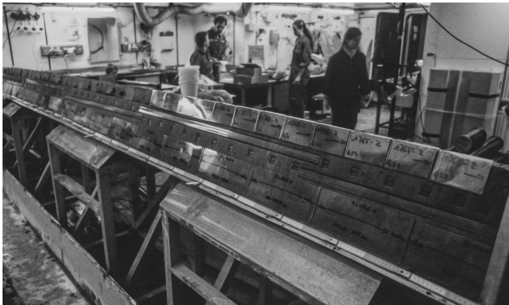
Figure 3: Sediment core taken with a Kastenlot (30 x 30 cm) prepared with Plexiglas lids to remove the samples for X-raying.
