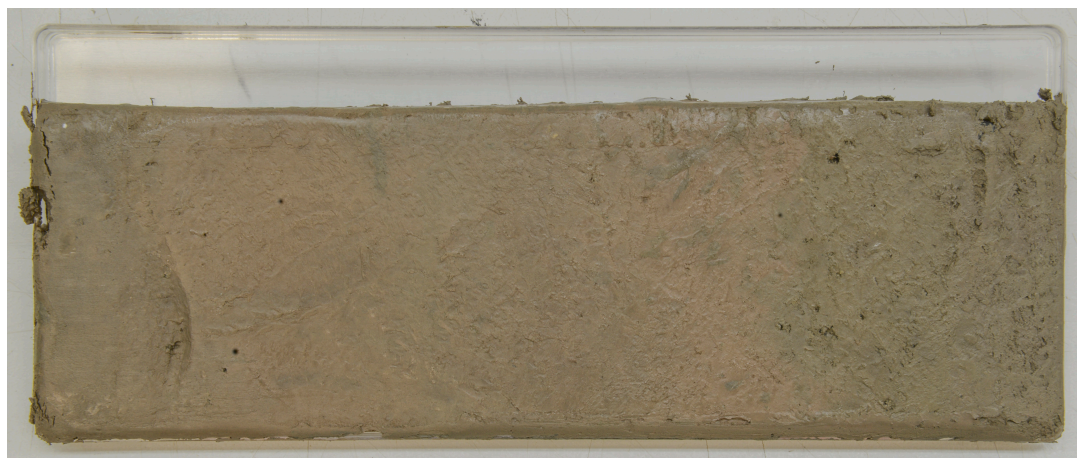
Figure 2: Sediment slab (25 x 10 cm) stabilized in plexiglas lid ready for X-raying.
