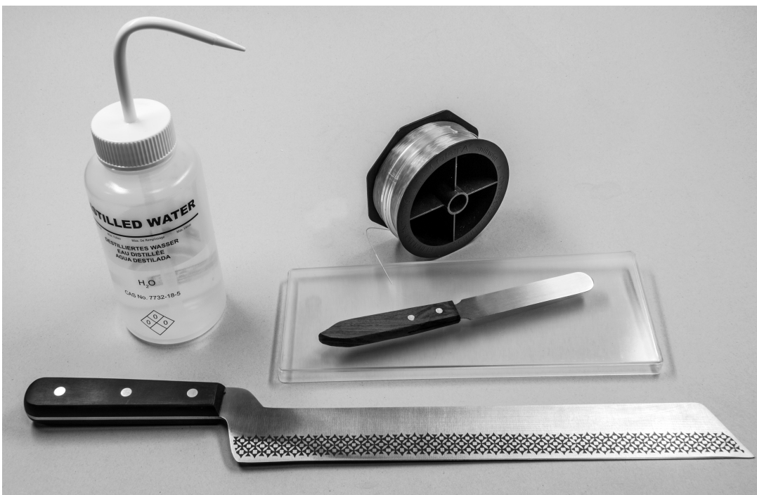
Figure 4: Equipment used for the preparation of sediment slabs for X-ray imaging comprise fishing line, distilled water, cheese knife, spatule and special Plexiglas lids for support of the sediment slab. Lids used for preparation have a size of 25 x 10 x 1 cm (Bensberger Kunststoffwerk Lappe GmbH).
