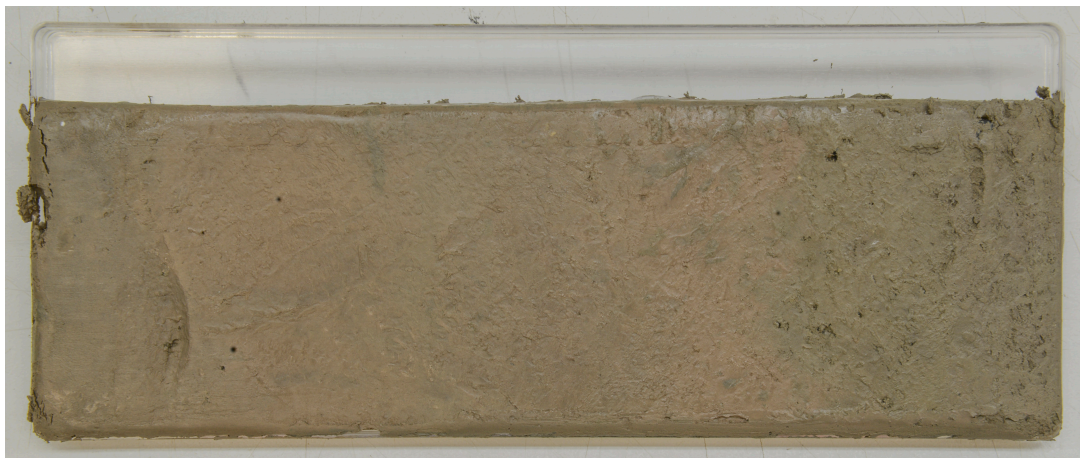
Figure 2: Sediment slab (25 x 10 cm) stabilized in plexiglas lid ready for X-ray imaging.
