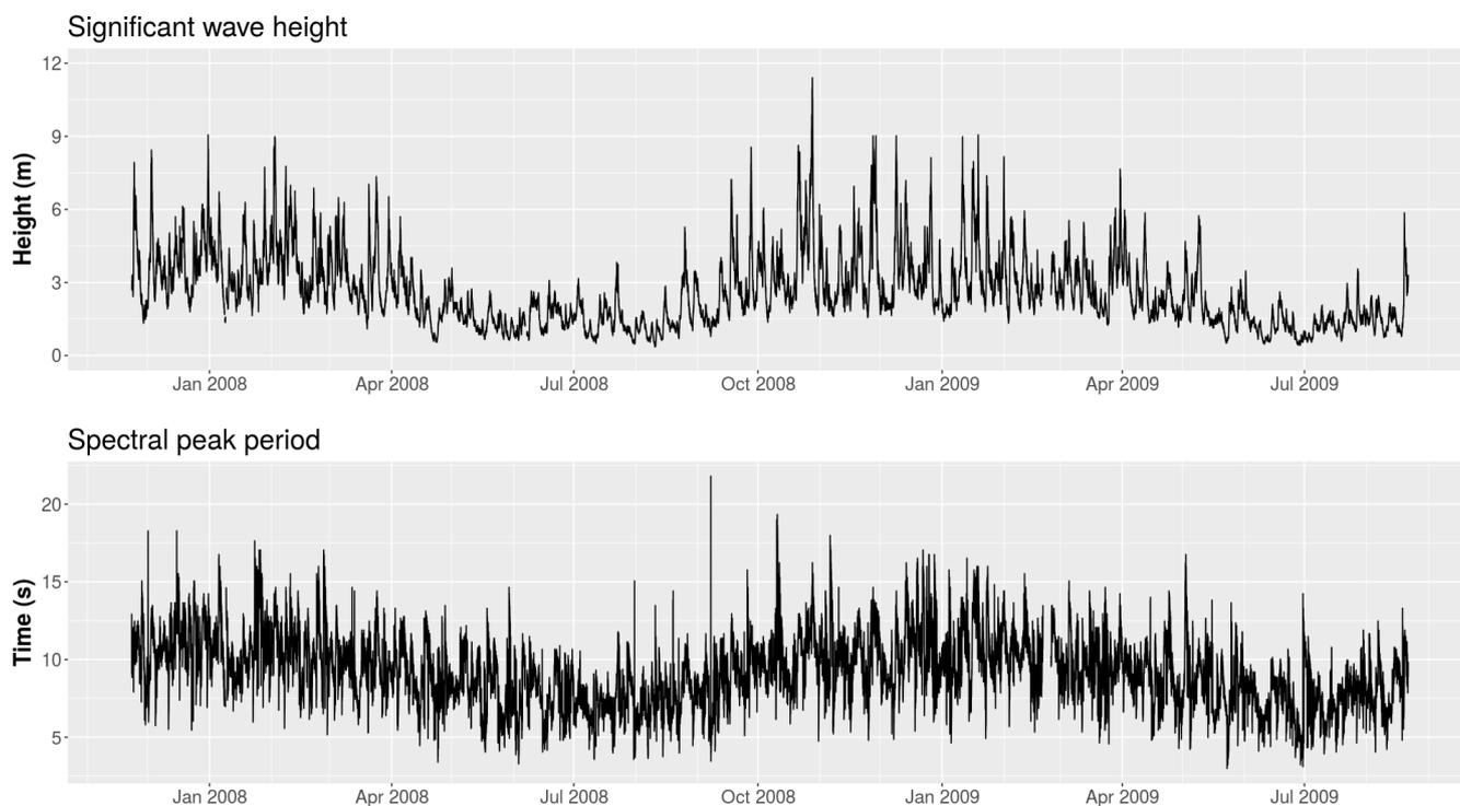
**Figure 12.** Measurements of significant wave height (m) and the spectral peak period (s).
