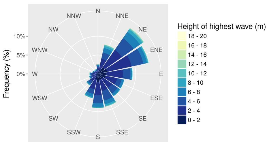
**Figure 11.** A frequency rose, showing the frequency (%) and height of highest wave (m) for different wave directions ( $22.5^\circ$  bins), with wave directions defined in the same way as wind directions.
