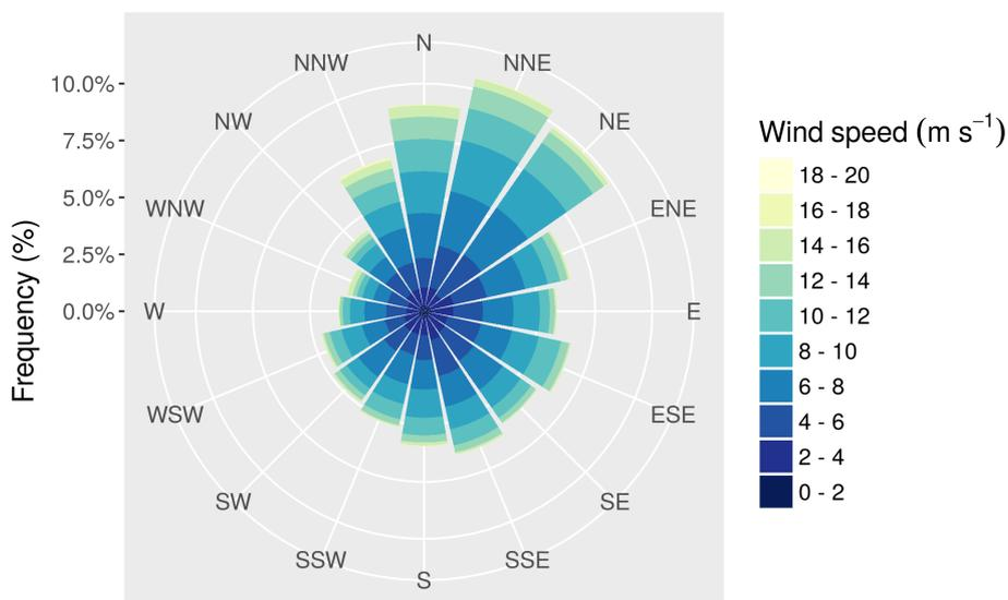
**Figure 6.** A wind rose, showing the frequency (%) and wind speed (m/s) for different wind directions at 4 m height (22.5° bins).
