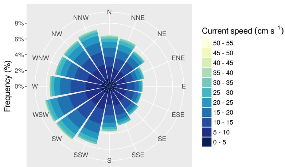
**Figure 10.** A frequency rose, showing the frequency (%) and current speed (m/s) for different current directions (22.5° bins) at 4 m height. Note that current direction is defined as the direction the current is streaming toward, which is opposite to the convention of wind direction.
