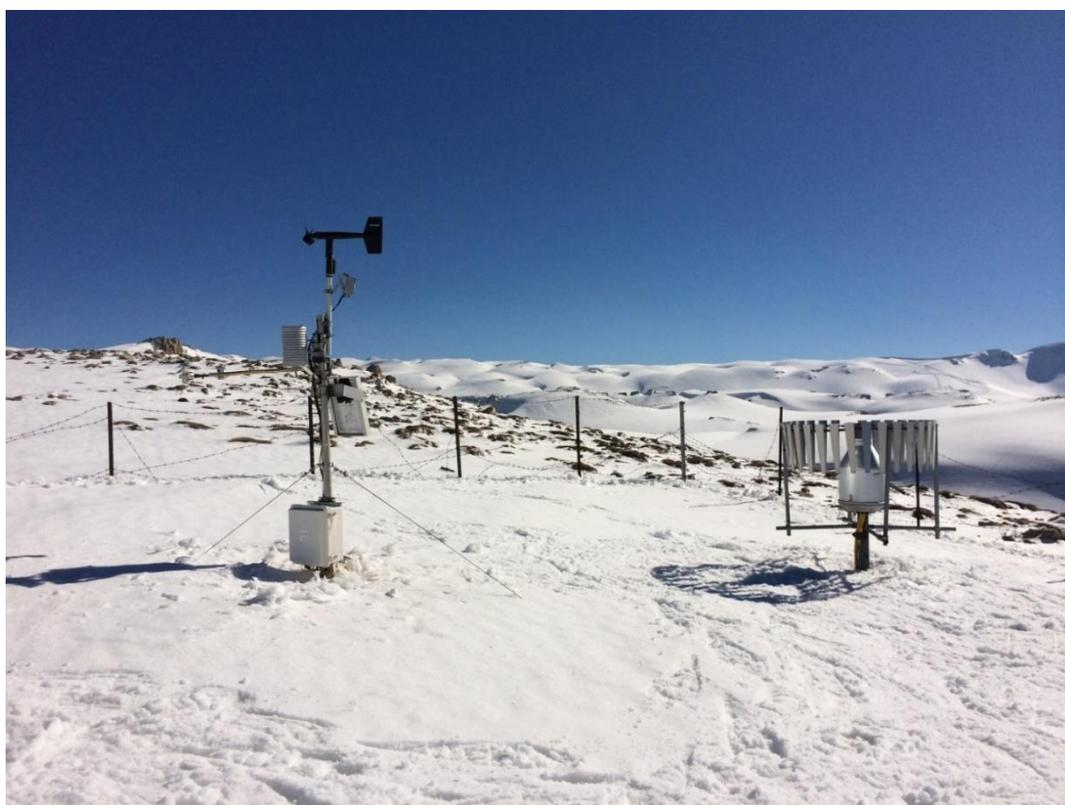
10 **Figure 3:** Automatic weather station at Mzar (MZA) (2296 m a.s.l.) where all sensors are located on the tower and the precipitation gauge is located to the right of the station. Image captured on March 5th, 2015 (courtesy of the author).
