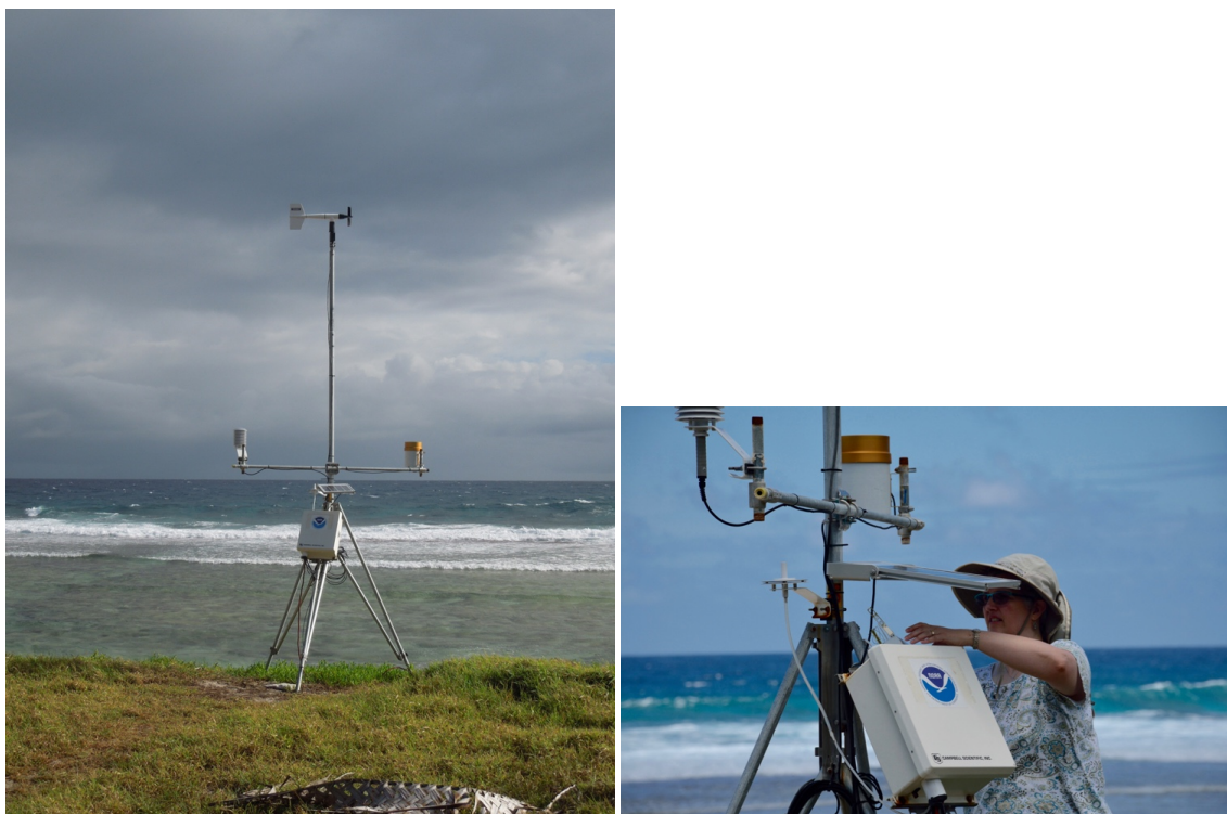
5 Figure 2: (a) The surface met station in its final position above the beach at Kiritimati. The anemometer sits atop the assembly, while the temperature/humidity sensor (left) and rain gauge (right) are attached to the crossbeam. Just below the crossbeam is the solar panel, and the box containing the Campbell datalogger, the power supply, and the barometer is mounted just below that. A plastic tube runs from the barometer out the tube on the bottom of the box, and can be seen mounted within a white disk just to the left of the solar panel. (b) The 26 March 2017 00 UTC radiosonde being put on the Campbell box in the shade of the solar panel prior to launch. The pressure tube egress and mount are clearly visible.
