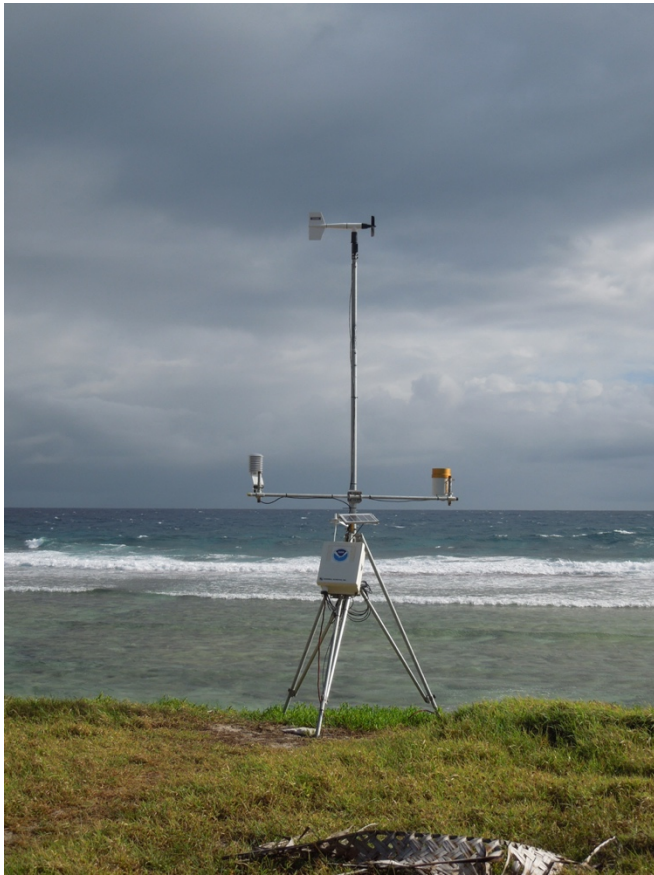
5 Figure 2: (a) The surface met station in its final position above the beach at Kiritimati. The anemometer sits atop the assembly, while the temperature/humidity sensor (left) and rain gauge (right) are attached to the crossbeam. Just below the crossbeam is the solar panel, and the box containing the Campbell datalogger, the power supply, and the barometer is mounted just below that. A plastic tube runs from the barometer out the tube on the bottom of the box, and can be seen mounted within a white disk just to the left of the solar panel. (b) The 26 March 2017 00 UTC radiosonde being put on the Campbell box in the shade of the solar panel prior to launch. The pressure tube egress and mount are clearly visible. Photo courtesy of G. Kerber.
