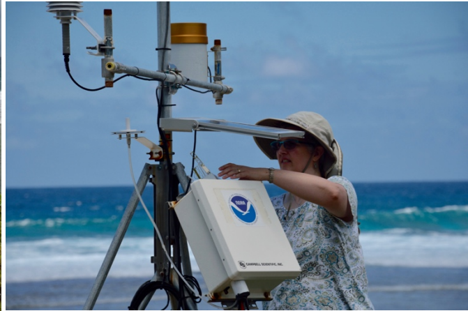
5 Figure 2: (a) The surface met station in its final position above the beach at Kiritimati. The anemometer sits atop the assembly, while the temperature/humidity sensor (left) and rain gauge (right) are attached to the crossbeam. Just below the crossbeam is the solar panel, and the box containing the Campbell datalogger, the power supply, and the barometer is mounted just below that. A plastic tube runs from the barometer out the tube on the bottom of the box, and can be seen mounted within a white disk just to the left of the solar panel. (b) The 26 March 2017 00 UTC radiosonde being put on the Campbell box in the shade of the solar panel prior to launch. The pressure tube egress and mount are clearly visible. Photo courtesy of G. Kerber.
