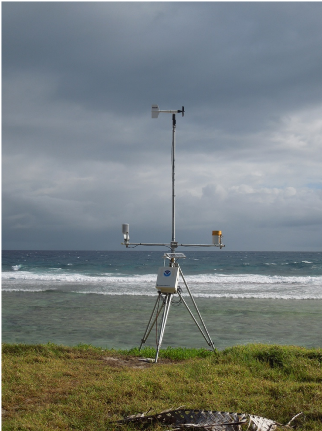
Figure 2: (a) The surface met station in its final position above the beach at Kiritimati. The anemometer sits atop the assembly, while the temperature/humidity sensor (left) and rain gauge (right) are attached to the crossbeam. Just below the crossbeam is the solar panel, and the box containing the Campbell datalogger, the power supply, and the barometer is mounted just below that. A plastic tube runs from the barometer out the tube on the bottom of the box, and can be seen mounted within a white disk just to the left of the solar panel. (b) The 26 March 2017 00 UTC radiosonde being put on the Campbell box in the shade of the solar panel prior to launch. The pressure tube egress and mount are clearly visible.
