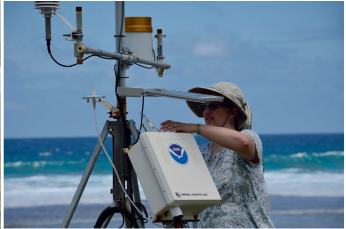
Figure 2: (a) The surface met station in its final position above the beach at Kiritimati. The anemometer sits atop the assembly, while the temperature/humidity sensor (left) and rain gauge (right) are attached to the crossbeam. Just below the crossbeam is the solar panel, and the box containing the Campbell datalogger, the power supply, and the barometer is mounted just below that. A plastic tube runs from the barometer out the tube on the bottom of the box, and can be seen mounted within a white disk just to the left of the solar panel. (b) The 26 March 2017 00 UTC radiosonde being put on the Campbell box in the shade of the solar panel prior to launch. The pressure tube egress and mount are clearly visible.
