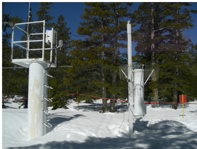
5 Figure 2. Sesame snow study site in April 2006. On the left is the tower where total snow depth is measured using a boom. On the right is a weighing gauge, manually raised and lowered about 1 m above the snow surface.
