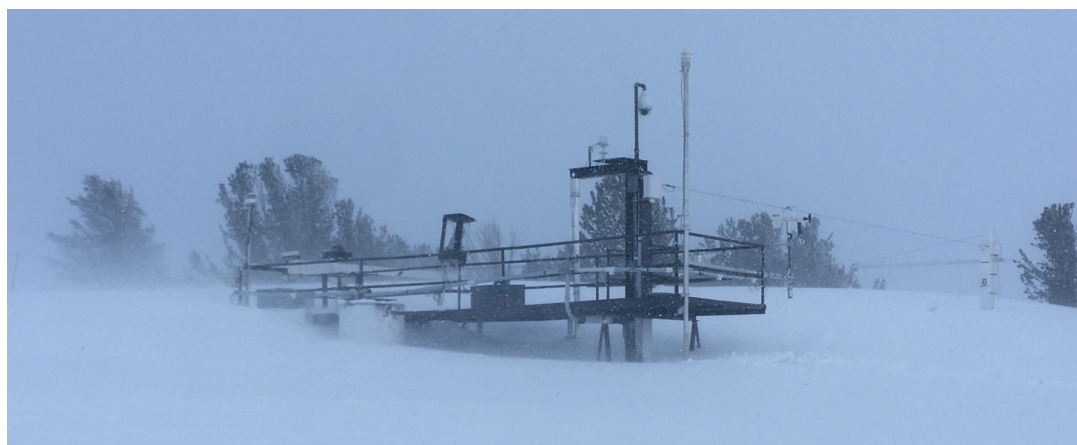
Figure 3. A nearly buried CUES platform in 2017 Feb. The RM Young 5103 is the white anemometer with a propeller. The SR50A is the downlooking silver sensor below. The snow depth has reached the CUES platform, 6 m above the ground, several times since 1987, but never completely buried it.
