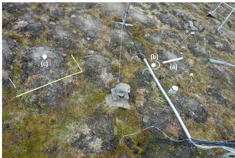
Figure C7. Soil profile and station location (a) 1998, (b) 1999, (c) 2009. Profile (b) upper temperature sensors were affected by reindeer disturbance in September 2003. Furthermore,
