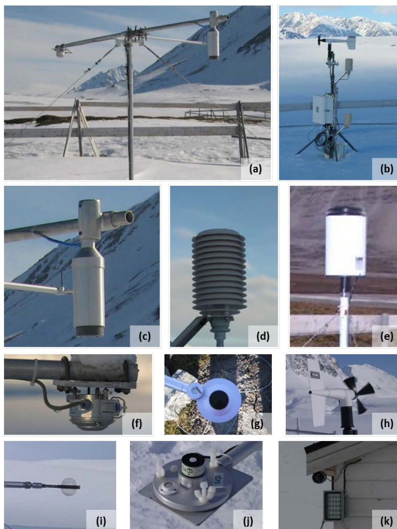
Figure C2. Climate station, Bayelva, Sept. 1998–Aug. 2009. (a) radiation/snow tower, (b) meteorological tower, (c) snowheight (from Sep 1999: 2 m. from Jul 2001, 1.6 m, from Sep 2003:1.45 m), (d) temperature/relative humidity (2 m) and temperature (1 m), (e) raingauge (1.68 m top of bucket above ground Level), (f) pyrgometer (from May 2003: 2 m; from Sep 2003: 2 m) installed in May 2002, (g) net radiometer (from Apr 2000: 1.14 m; from Sep 2003: 1.6 m), (h) windspeed/-direction (3 m), (i) net radiation (from Apr 2000:1.14 m, from Sep 2003: 1.6 m), (j) pyranometer (2 m), (k) camera (2 m) with flash since Aug 2013; sensor details can be found in Table 2.
