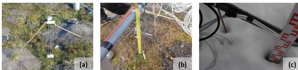
Figure C5. (a) Vertically installed time-domain reflectometry (TDR) air/ snow TDR probe (50 cm length) above the ground surface during summer at the Bayelva climate station (1999). During winter (fully snow covered), the dielectric number of snow is recorded. (b) PT100 temperature sensors in air (summer) at 4 and 20 cm above ground surface, (c) PT100
