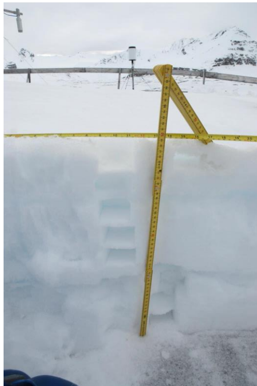
Figure E112. Snow profile taken on 9 May 2016, inside the Bayelva fenced area. The pockets/holes are the result of snow removal using a snow density cutter ( 100 \text{ cm}^3 ). Snow
