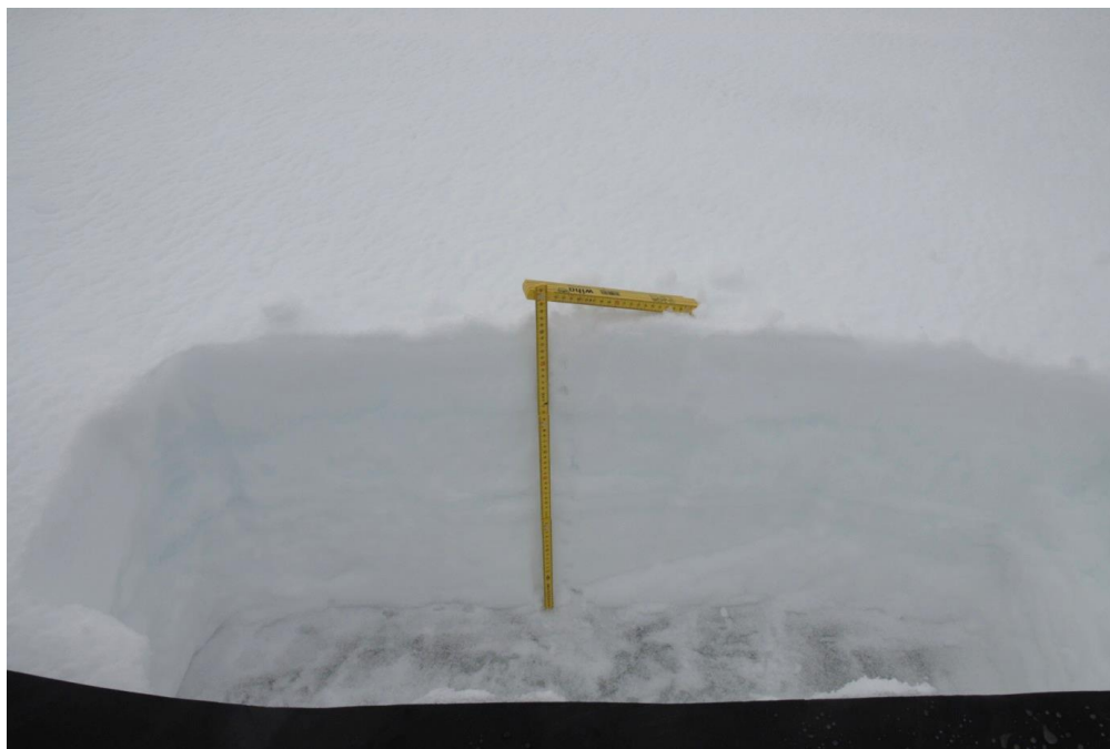
Figure E213. Snow pit, 10 May 2016. The basal ice layer is visible at the bottom of snow layer. Two profiles were measured one to the left and one to the right from the yellow meter stick (profile data named left and right in Table E1). Further data on temperatures, dielectric numbers, and stratigraphy can be found in table E1.
