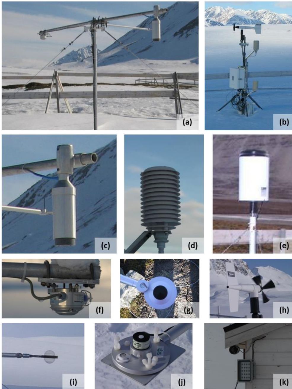
Figure C2. Climate station, Bayelva, Sept. 1998–Aug. 2009. (a) radiation/snow tower, (b) meteorological tower, (c) snowheight (from Sep 1999: 2 m. from Jul 2001, 1.6 m, from Sep 2003:1.45 m), (d) temperature/relative humidity (2 m) and temperature (1 m), (e) raingauge (1.68 m top of bucket above ground Level), (f) pyrgeometer (from May 2003: 2 m; from Sep 2003: 2 m) installed in May 2002, (g) net radiometer (from Apr 2000: 1.14 m; from Sep 2003: 1.6 m), (h) windspeed/-direction (3 m), (i) net radiation (from Apr 2000:1.14 m, from Sep 2003: 1.6 m), (j) pyranometer (2 m), (k) camera (2 m) with flash since Aug 2013; sensor details can be found in Table 2.
