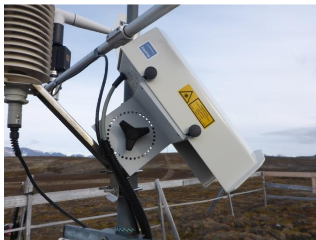
Figure C4. Laser snow depth sensor attached to the climate station, Bayelva, Aug. 2013–present, UTM: 33 N 432100 8762992.
