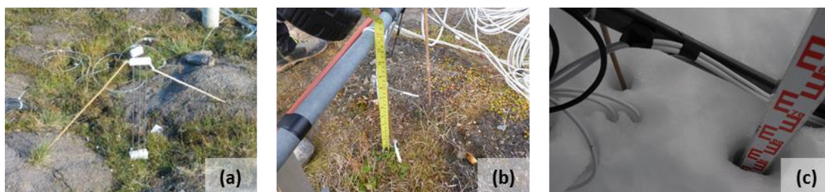
Figure C5. (a) Vertically installed time-domain reflectometry (TDR) air/ snow TDR probe (50 cm length) above the ground surface during summer at the Bayelva climate station (1999). During winter (fully snow covered), the dielectric number of snow is recorded. (b) PT100 temperature sensors in air (summer) at 4 and 20 cm above ground surface, (c) PT100 temperature sensors in air (summer) at 4 and 20 cm above ground surface.
