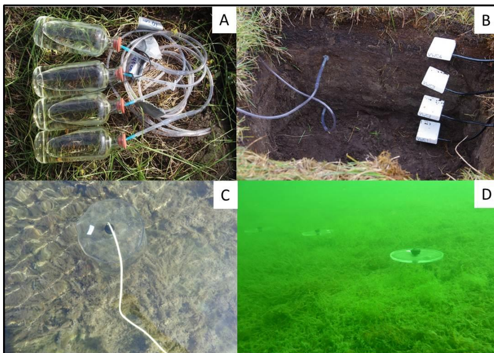
Figure 5. Photos of lysimeter flasks (A), lysimeter installation (B), and respiration chambers for benthic production/respiration measurements (C and D).
