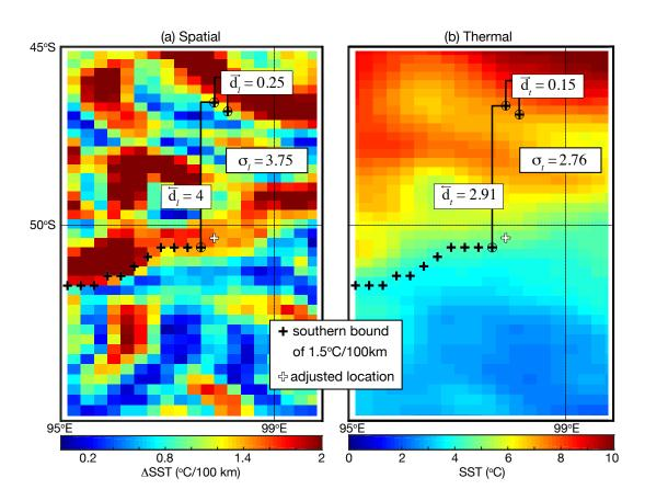
**Figure 1.** Example of (a) spatial and (b) thermal discontinuity resulting in an adjustment in the PF location according to (1) as outlined in Section 2.2.2.
