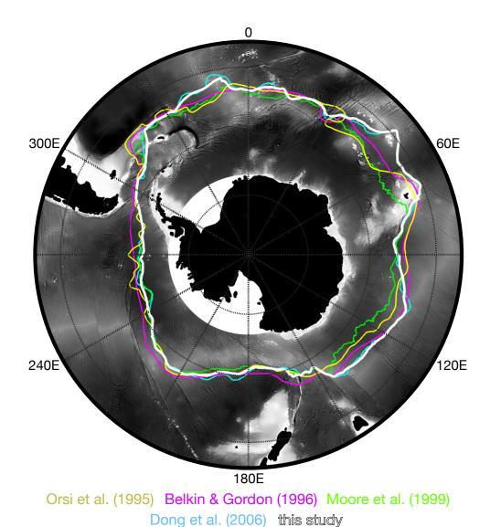
**Figure 6.** The climatological position of the PF in this and previous studies overlain on bottom topography, where light (dark) shading indicates shallow (deep) bathymetry.
