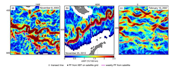
Figure 3. PF location identified from surface XBT data (timestamp indicated) overlain on the corresponding weekly satellite-estimated  $\Delta$ SST and PF realization in the (a) Australian, (b) Drake Passage, and (c) African sectors.
