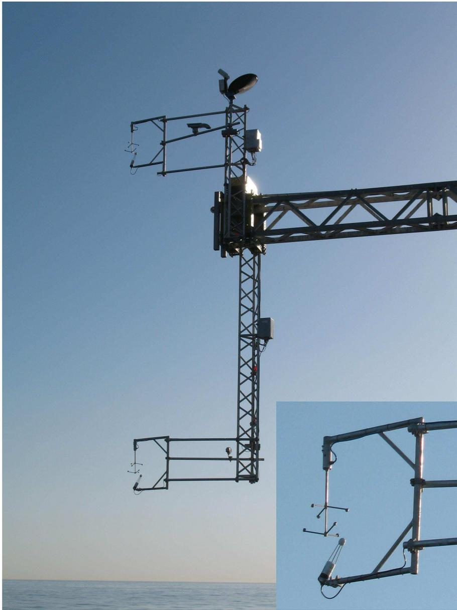
**Figure 2.** Instrument boom at FINO2 with the turbulence sensors at both heights and instrument installation in more detail (small picture).
