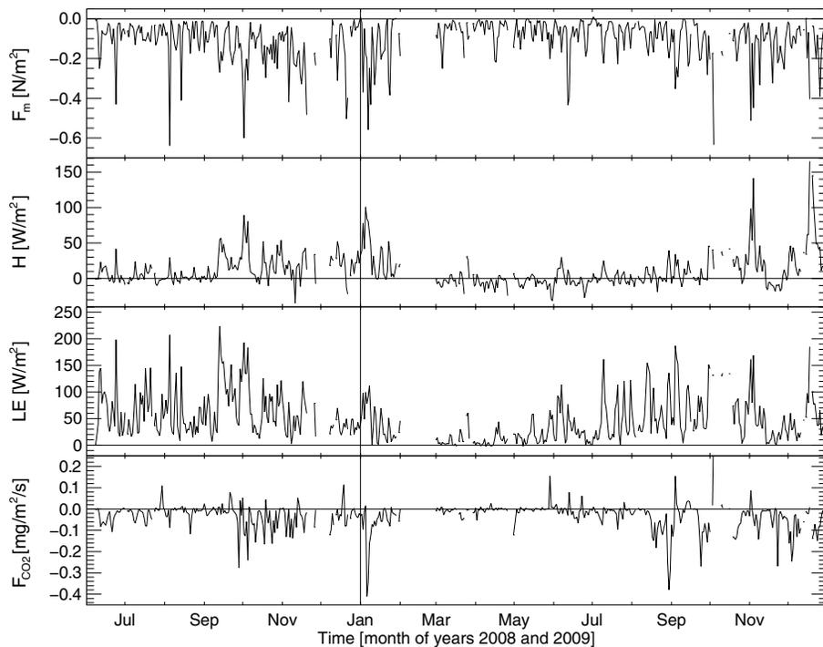
**Figure 3.** Daily means of momentum flux  $F_M$ , sensible and latent heat flux,  $H$  and  $LE$ , and  $CO_2$  flux in 13.8 m height, from June 2008 to December 2009.
