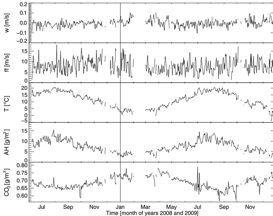
**Figure 2.** Daily means of measured quantities at 13.8 m height above sea surface: vertical wind speed  $w$ , horizontal wind speed  $ff$ , air temperature  $T$ , absolute humidity  $AH$ , and CO<sub>2</sub> density from June 2008 to December 2009.
