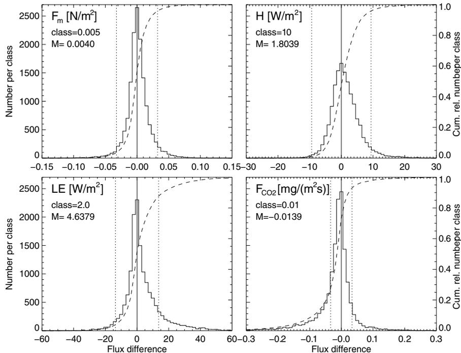
**Figure 5.** Distribution of flux differences (TOP-BOTTOM) for momentum ( $F_m$ ), sensible ( $H$ ) and latent heat ( $LE$ ), and CO<sub>2</sub> flux ( $CO_2$ ), based on 30 min values for 1.5 years.  $M$  gives the mean difference, class stands for the width of class for each flux difference. The dotted lines give the measurements uncertainties, derived from the RMSE.
