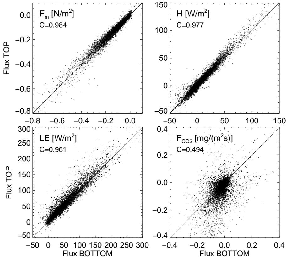
**Figure 4.** Comparison of turbulent fluxes at two different heights, TOP (13.8 m) vs. BOTTOM (6.8 m). The temporal resolution is 30 min. Top: momentum flux  $F_m$  (left) and sensible heat flux  $H$  (right), bottom: latent heat flux  $LE$  (left) and CO<sub>2</sub> fluxes (right).  $C$  gives the correlation coefficient.
