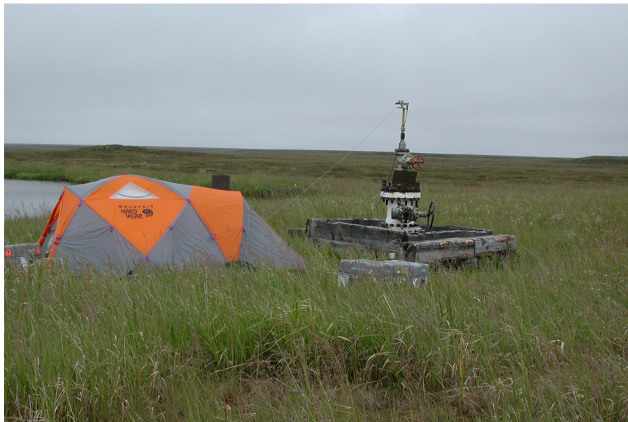
Fig. 3. Measuring temperatures in the Koluktak (KOL) Test Well No. 1, National Petroleum Reserve–Alaska. This well is typical of the other wells in the DOI/GTN-P Borehole Array.
