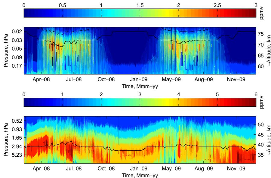
**Fig. 4.** Top panel: BAS-MRT ozone data showing the mesospheric ozone. The solid black line indicates the upper limit of the 0.8 measurement response, while the dashed black line indicates the upper limit of 0.5 measurement response. Bottom panel: stratospheric ozone observations from BAS-MRT. The solid black line indicates the lower limit of 0.8 measurement response.
