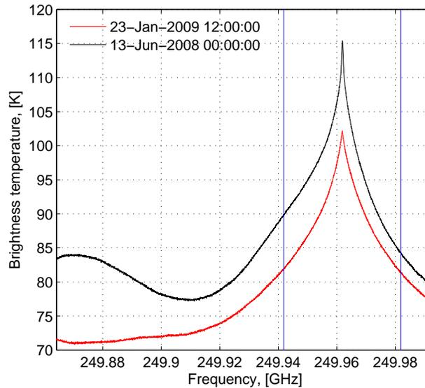
**Fig. 2.** Noon summer (red) and midnight winter (black) calibrated atmospheric spectra. The blue vertical lines indicate the frequency range of the spectra used in the  $O_3$  retrieval.
