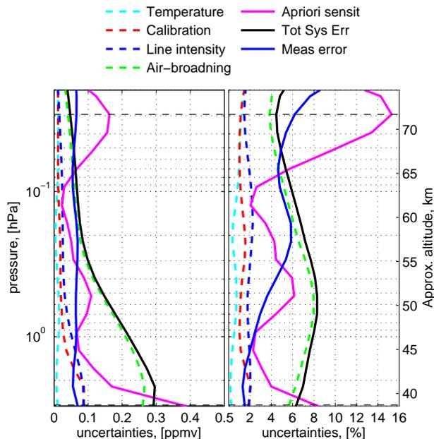
**Fig. 5.** Error estimations of the BAS-MRT  $O_3$ -retrieval: the black solid line shows the total systematic error, which is the root-sum-square of the dashed lines. The blue solid line is the random measurement error. The magenta solid line is the a priori sensitivity. Dashed horizontal black lines indicate the upper/lower limit of the 0.8 measurement response. Left panel: uncertainties in ppmv representing all times. Right panel: uncertainties in % of midnight  $O_3$ -profile.
