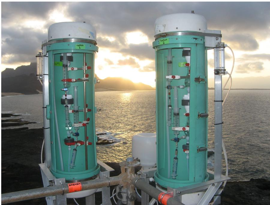
**Fig. 3.** Mist chambers at the Cape Verde sampling tower.
