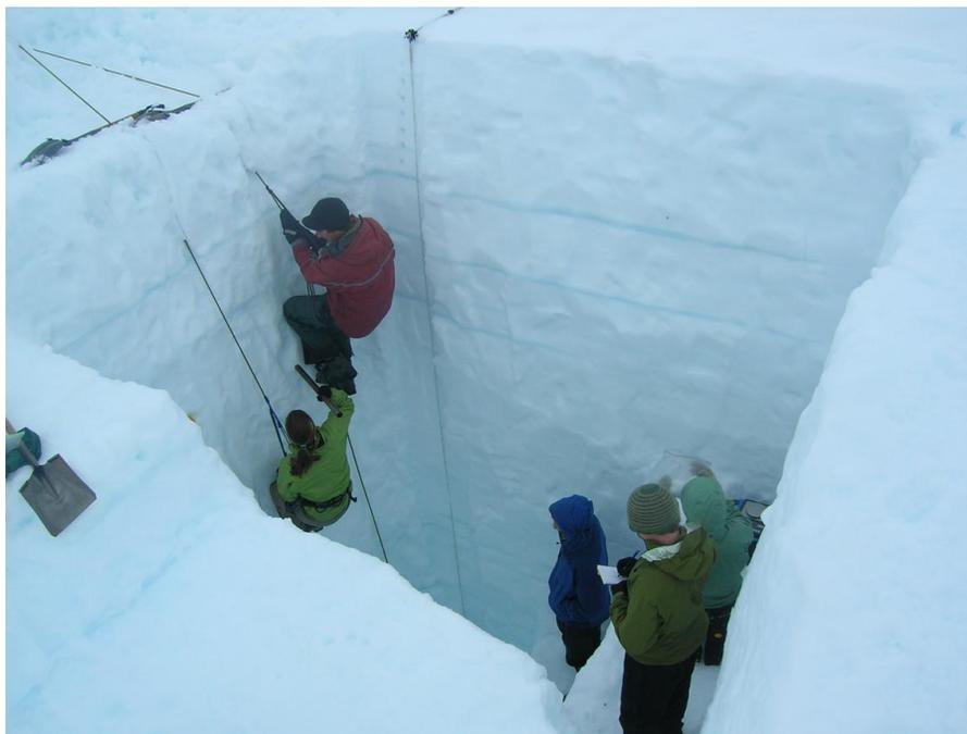
**Fig. 3.** Snowpit on Taku Glacier in 2011. Note the ice lenses. Density measurements are being taken from the south wall; the tape measure aids recording ice lens and sample depths.
