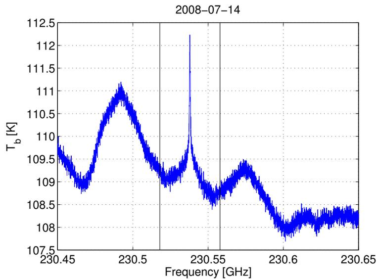
**Fig. 2.** Calibrated spectrum before tropospheric correction. The solid black vertical lines mark the part of the spectrum used for the profile retrieval.
