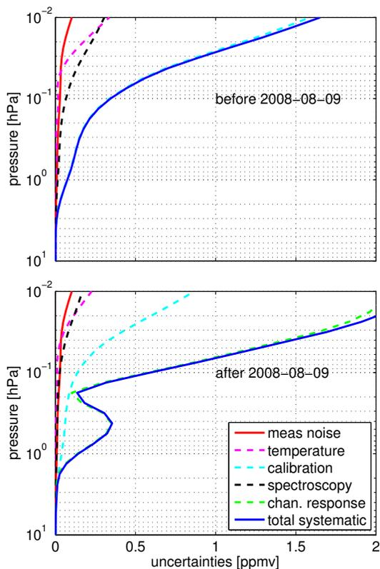
**Fig. 6.** Estimated uncertainties for the BAS radiometer. The uncertainty caused by the measurement noise ( $1\text{-}\sigma$ , red) is regarded as random while the systematic error ( $2\text{-}\sigma$ ) is determined by perturbing the temperature profile (magenta dashed), calibration (cyan dashed), spectroscopic parameters (blue dashed) and the channel response function (green dashed) with the respective uncertainties. Top: before 9 August 2008, Bottom: after 9 August 2008.
