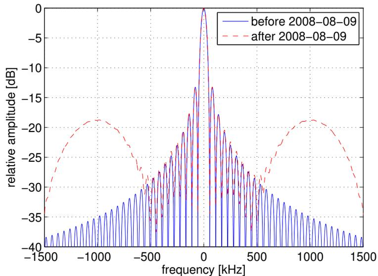
**Fig. 4.** Channel response functions used in the retrieval before and after 9 August 2008.
