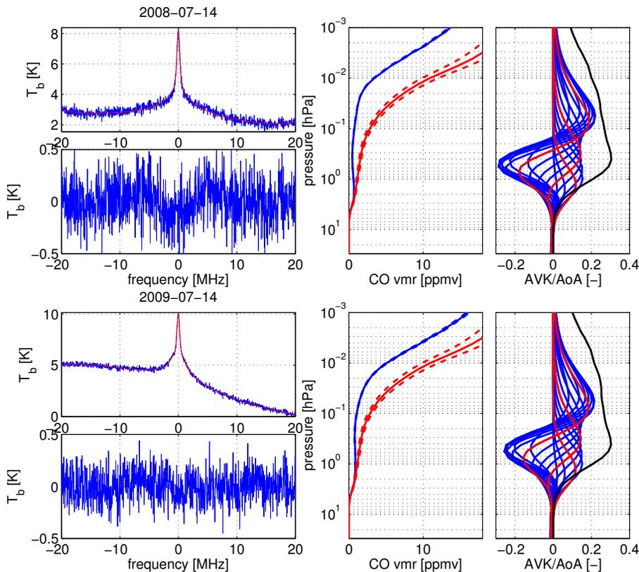
**Fig. 5.** Retrieval before (top) and after (bottom) 9 August 2008. Left top: calibrated spectrum after tropospheric correction (blue) and fit found using optimal estimation (red). Bottom left: residuals. Middle: estimated atmospheric profile with measurement error (blue) and a priori with covariance (red). Right: AVK (red – 1, 0.1 and 0.01 hPa) and area of the AVK divided by 4 (measurement response).
