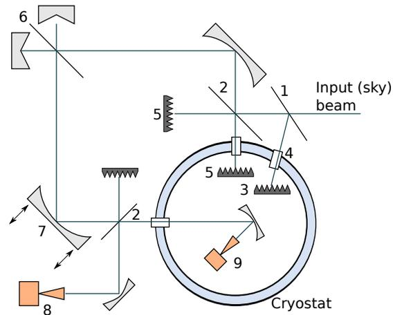
**Fig. 1.** Schematic drawing of the heterodyne receiver of the BAS microwave radiometer.
