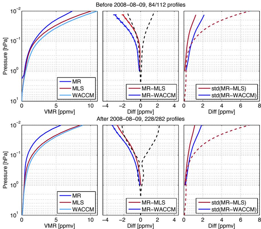
**Fig. 8.** Intercomparison between BAS microwave radiometer (MR) and MLS (red) or SD-WACCM (light blue), respectively. Left: mean coincident profiles of BAS radiometer (blue), MLS and SD-WACCM. Middle: bias with standard error and estimated systematic error of the BAS radiometer. Right: standard deviation of difference and combined random errors of MLS and the BAS radiometer (red dashed).
