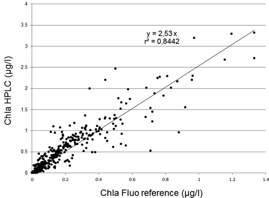
**Fig. 3.** Relationship between the chl *a* concentration provided by the reference fluorometer and the Chlorophyll *a* concentration estimated from HPLC measurements. This relationship was estimated over 70 test profiles ranging between 30 to 200 m and performed between 2002 and 2009.
