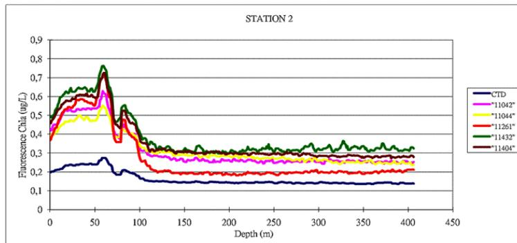
**Fig. 2.** Example of fluorescence profiles provided by different CTD-FLUO-SRDs and the reference fluorometer (in blue) obtained at two different stations. These profiles exhibit the existence of a fluorescence offset differing between CTD-FLUO-SRDs. Fluorometers were providing consistent data between each other but differed in the absolute amount of fluorescence produced.
