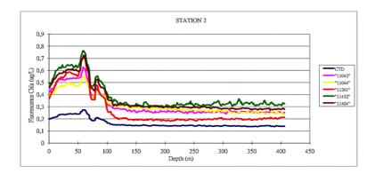
Fig. 2. Example of fluoresecence profiles provided by different CTD-FLUO-SRDLs and the reference fluorometer (in blue) obtained at two different stations. These profiles exhibit the existence of a fluorescence offset differing between CTD-FLUO-SRDLs. Fluorometers were providing consistent data between each other but differed in the absolute amount of fluorescence produced.
