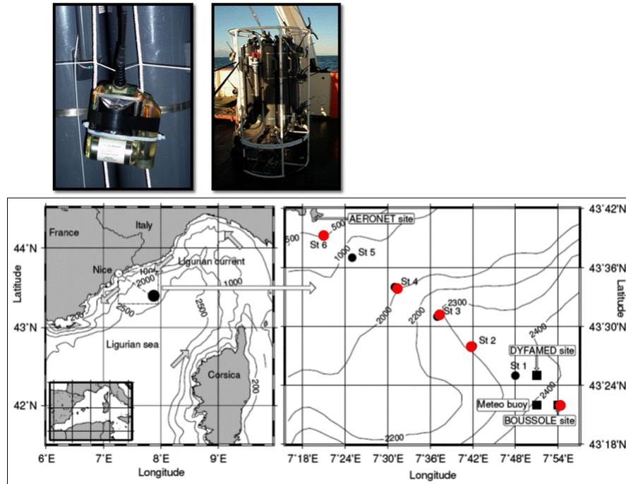
**Fig. 1.** Top: CTD-FLUO-SRDL were fixed on the external part of the CTD-cage. Bottom: the Boussole at sea test set up. Fluorescence profiles were conducted on stations located on the transect between Villefranche sur mer and the BOUSSOLE site (right). A fluorescence profile combined with water sampling for HPLC assessment of Chlorophyll *a* concentration was performed at the BOUSSOLE site located 70 miles off Villefranche sur mer (left).
