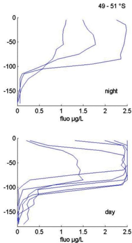
**Fig. 6.** Example of unquenched night fluorescence profiles (top) and quenched day ones (bottom) collected on the same location and same period by a CTD-FLUO-SRDL deployed on a male SES foraging over the Kerguelen plateau.
