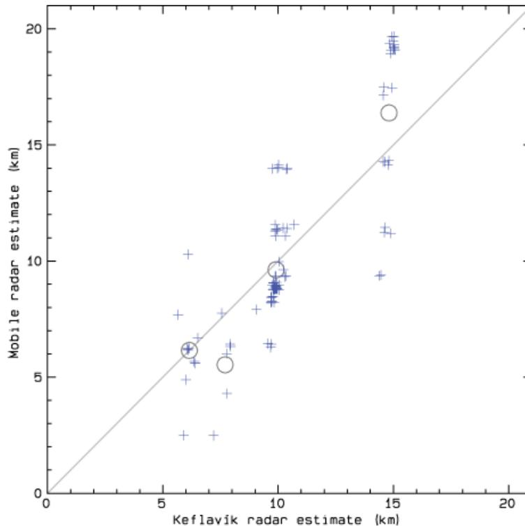
**Fig. 6.** Comparison of synchronous plume-top altitude estimates by the two radars. The circles show mean values of clusters for the Keflavík radar elevation angles, see Table 3.
