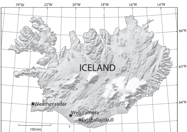
Figure 1. A map of Iceland and the location of the weather radar at Keflavik airport, the web camera in the village of Hvolsvöllum and the Eyjafjallajökull volcano in South Iceland. The radar is about 155 km from the volcano and in between there is a mountain range that obstructs the view of the plume when below 2.9 km a.s.l.
