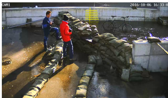
Figure 7. View from camera CAM1 in which a bicycle is visible in the flood water behind the dam. Deep learning could make it possible to automatically estimate the water level from such an image. An ultrasonic sensor above the water and a pressure sensor in man-hole m1 provide water level data.
