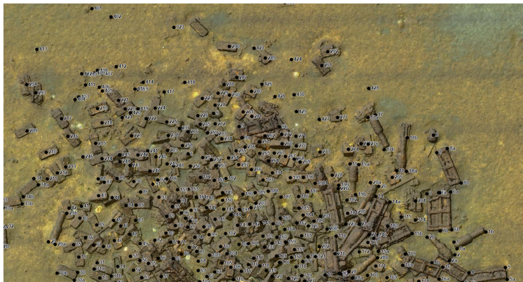
Figure 2. Example part of an annotated photomosaic. The figure shows the northern half of munition pile Haf_00318 as annotated by expert 1. Numbers with lowercase letters indicate objects that were measured in two dimensions (e.g., objects 1 and 8 in the east). The expert counted 483 objects and measured 52 of them, with the largest one measuring 1.24 m in length (© 2026 DSM, GEOMAR).
