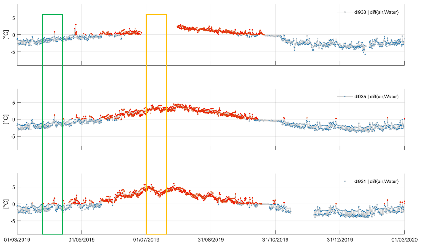
Figure 10. The difference between the sewer headspace temperature and the bulk liquid temperature observed at three specific locations in the main collector. Red dots indicate periods of evaporation (higher temperature in the headspace compared to the bulk liquid) and blue colours indicate periods of condensation (inverse temperatures). From the Supplement of Figueroa et al. (2021).
