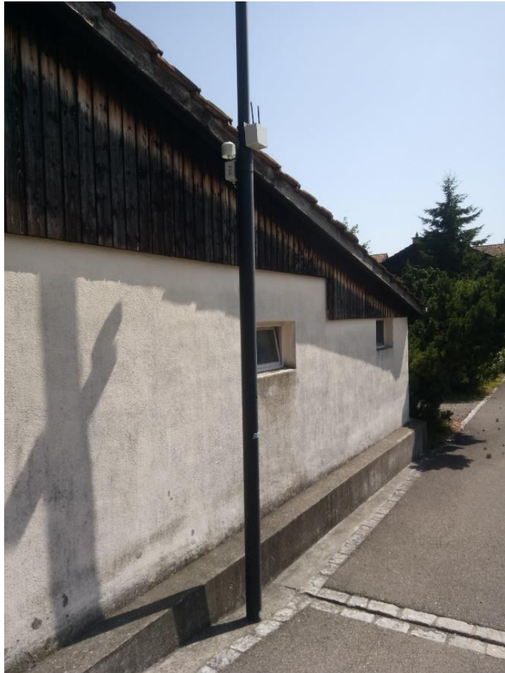
Figure S26. Ambient temperature and humidity sensor mounted at a lamp pole (backside).
