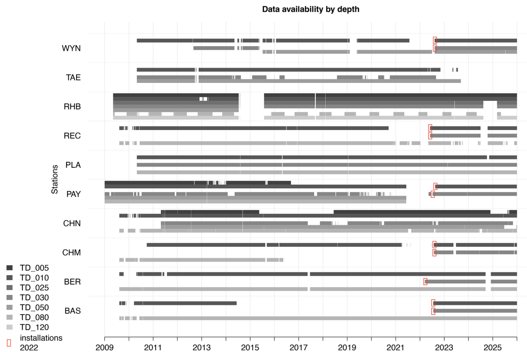
Figure 2. Time series diagram of the IMKO TRIME-PICO TDR (TD) sensor availability at the SwissSMEX grassland stations on the Swiss Plateau. Abbreviations for station names are given in Table 1; numbers alongside the sensor type indicate the installation depth in cm. This is a condensed view that combines all redundant sensor profiles. Note that station RHB includes an additional sensor at 25 cm depth, and that the sensors at the other depths are partly shifted by 5 cm in this profile. For simplicity, the sensors installed at depths of 15, 35 and 55 cm are shown as TD_010, TD_030, and TD_050, respectively. The TDR installations in 2022 are highlighted by red rectangles.
