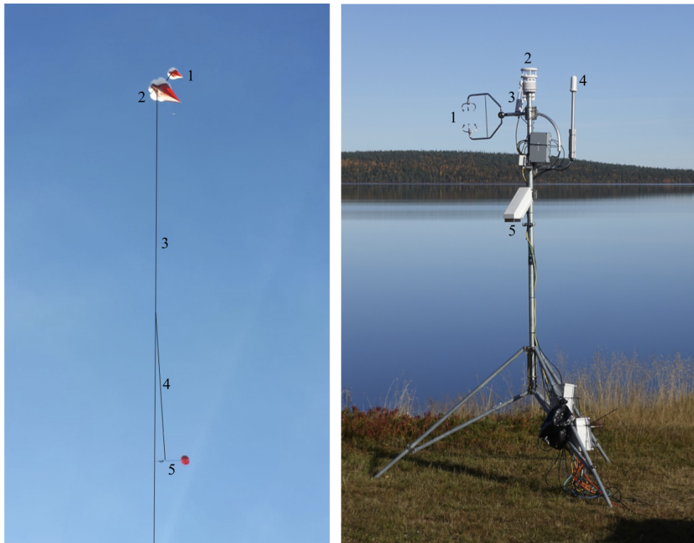
Figure 3. (Left) The Helikites of the MPCK platform (1, 2) lift a WinDart (5), which is connected to a line (4) and stabiliser, both attached to the main tether of the MPCK platform (3). (Right) The ground weather station with its main components: (1) Metek uSonic3 Class A-MP anemometer, (2) Lufft WS500UMB weather station including pressure, temperature, humidity and 2D wind velocity sensor, (3) Li-Cor LI-7500DS fast trace gas and humidity sensor, (4) Boltek LD-250 lightning detector, and (5) Campbell Scientific CS110 electric field meter.
