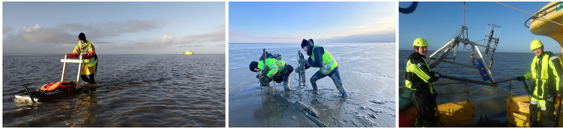
Figure 2. Photographs illustrating the installation of the measurement stations. Left: transport of instruments and equipment to intertidal measurement locations, after vessel grounding. Middle: in situ assembly of a scaffold frame equipped with instruments on a fringing mudflat. Right: deployment of an instrumented lander from a vessel.
