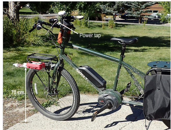
Figure A1. Surly Big Easy electric-assist bicycle with sensor package mounted on front rack. A fully-charged battery supported 80–90 km of lowest level (“Eco” mode) assist. In general, rides northbound involved slight descents, requiring little or no battery assist. Rides southbound typically involved slight ascent generally at second-level (“Tour”) assist. I never exhausted battery assist capacities. Sensors sat 70 cm above ground surfaces. Sensor box derived power from USB tap on rear of headlight.
