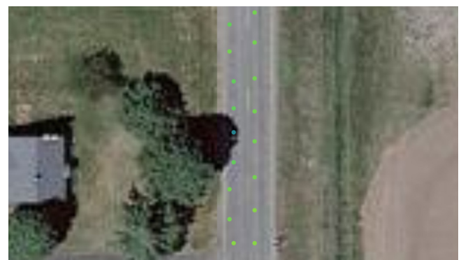
Figure 18. Data from CW and CCW Fowler loop rides on 30 June 2022, demonstrating shade-induced cool surface temperatures measured during CW loop (left track along west lane) followed (less than 20 min later) by identical but non-shaded measurements during CCW loop (right track along east lane). Image based on identical temperature scales northbound and southbound. Data clearly demonstrate cooling impact extending part-way across road surface during southbound pass while northbound pass – without shade – shows no impact. (Particular Google Earth image as GIS background, recorded under very similar late-day insolation conditions, tends to emphasize this pattern.) Background data © Google Earth.
