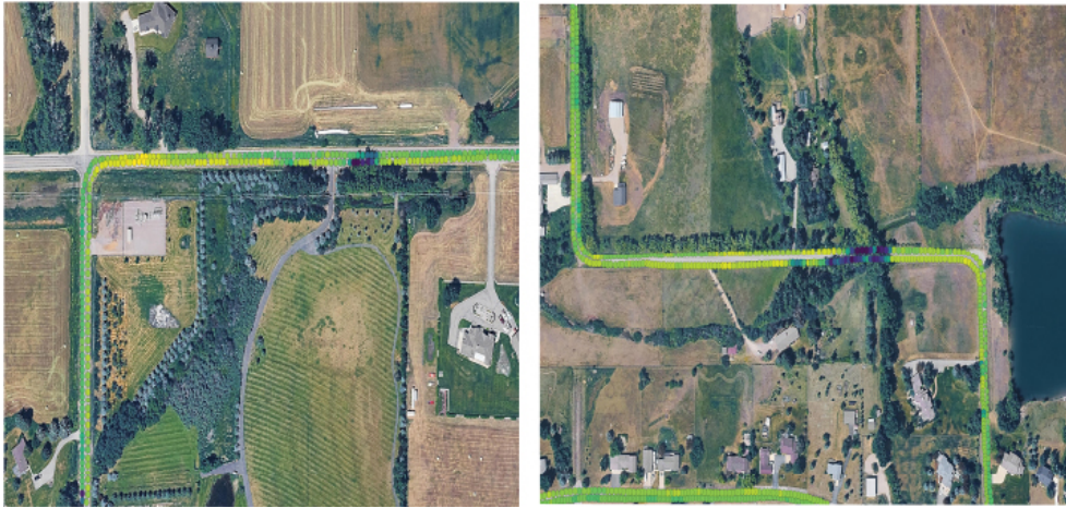
Figure 13. Surface temperatures minus air temperatures ( = T_{\text{sfc}} - T_{\text{air}} ) for rides clockwise starting at 73 269 s UTC ( \sim 13:35 local time) then counter-clockwise starting immediately after at 76247 s UTC ( \sim 14:18 local time), around Fowler loop on 30 June 2022. Data (color) scales, (particularly for temperature maximum) nearly identical in both cases (see also Table 1). In each plot, upper track in east-west direction records data from second counter-clockwise ride. In all cases, location of maximum surface warming ( T_{\text{sfc}} - T_{\text{air}} > 30^\circ\text{C} ) occurred close to patches of cooler surface temperatures in “permanently” shaded areas. Background data © Google Earth.
