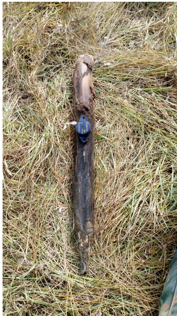
Figure D1. Proges Plus Thermo Buttons 22L (TB) attached on wooden peg. Installation by pushing or hammering into the soil to a depth of approximately 5 cm.
